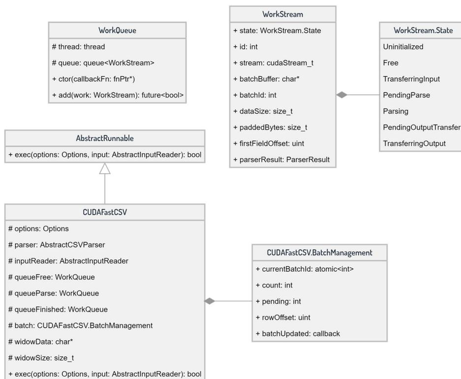
Figure 30: UML class diagram of components that act as a facade for CUDA Fast CSV
