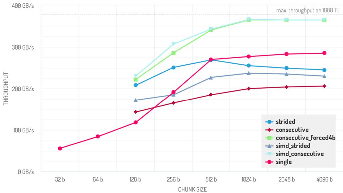
Figure 33: Throughput for chunk size with various access patterns on GTX 1080 Ti
