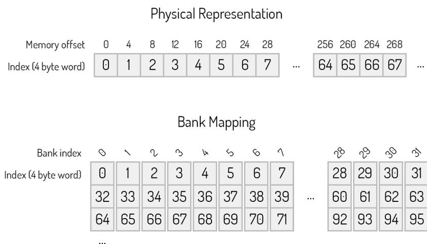
Figure 11: Mapping physical bytes to shared memory bank indexes
