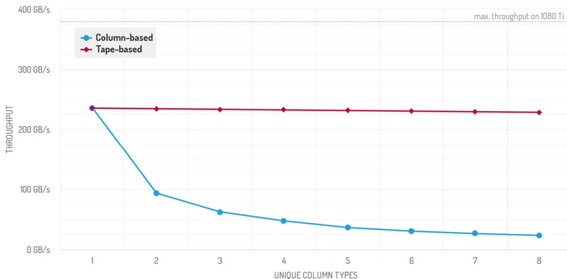
Figure 35: Column-based vs tape-based deserialization performance scaling on GTX 1080 Ti
