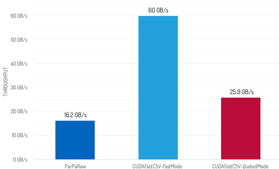
Figure 43: Comparing on-GPU throughput of ParPaRaw to CUDAFastCSV
