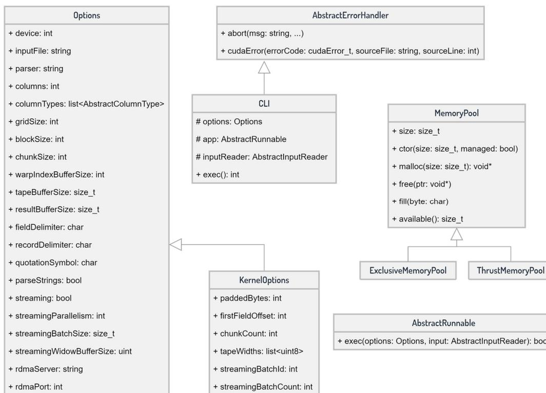
Figure 27: UML class diagram of helper components used throughout CUDA FastCSV
