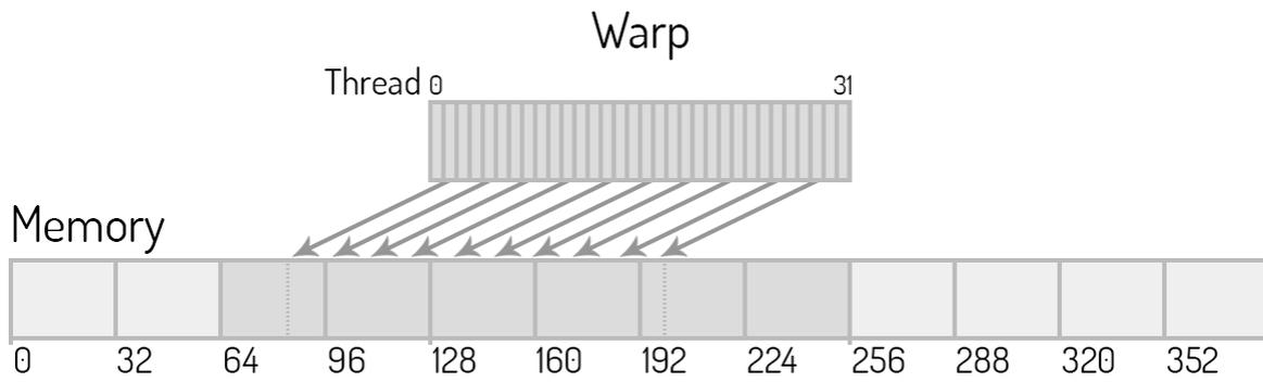
Figure 8: *Coalesced* but misaligned access. Warp requests 32 consecutive 4 byte elements but not from a 128 byte aligned address. The addresses fall within at most five sectors but six sectors are loaded. Bus utilization is 66.67%.
