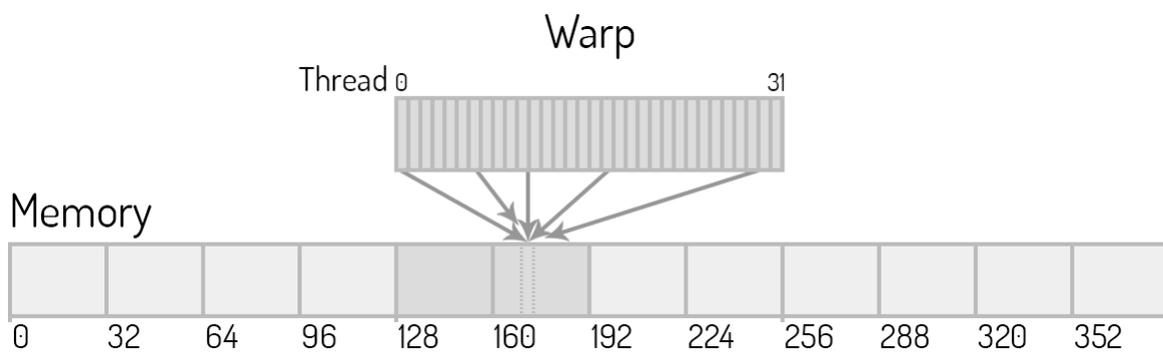
Figure 9: All threads in warp request same 4 byte data. The addresses fall within one sector but two sectors are loaded. Bus utilization is merely 6.25%.
