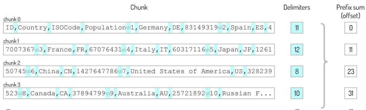
Figure 18: Computing the field offset for every chunk using a prefix sum
