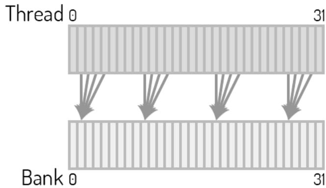
Figure 14: Irregular access pattern. Several bank conflicts with multiple threads accessing the same bank. Conflict-free broadcast access only possible if threads access the same address within the bank. Poor bandwidth utilization.
