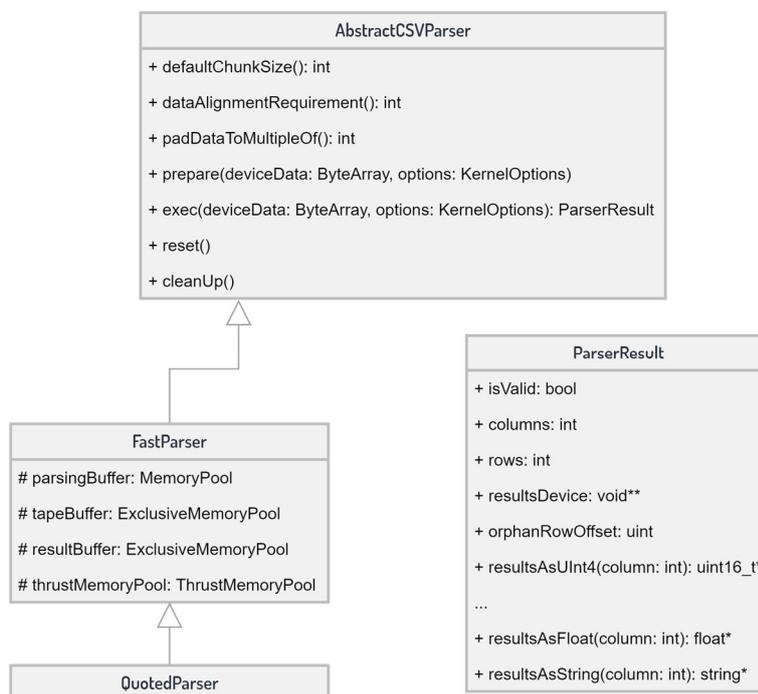
Figure 28: UML class diagram of components relevant to parsing
