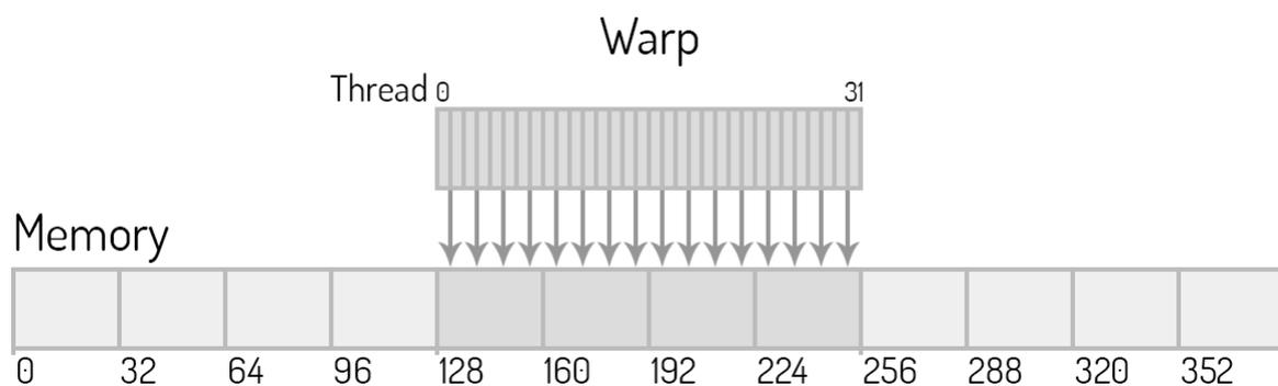
Figure 7: Ideal case, *aligned* and *coalesced* access. Addresses required for the 128 bytes requested fall within four sectors. Bus utilization is 100% with no loads wasted.
