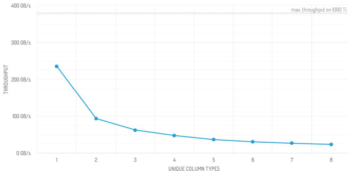
Figure 22: Column-based deserialization performance scaling for unique data types on 1080 Ti
