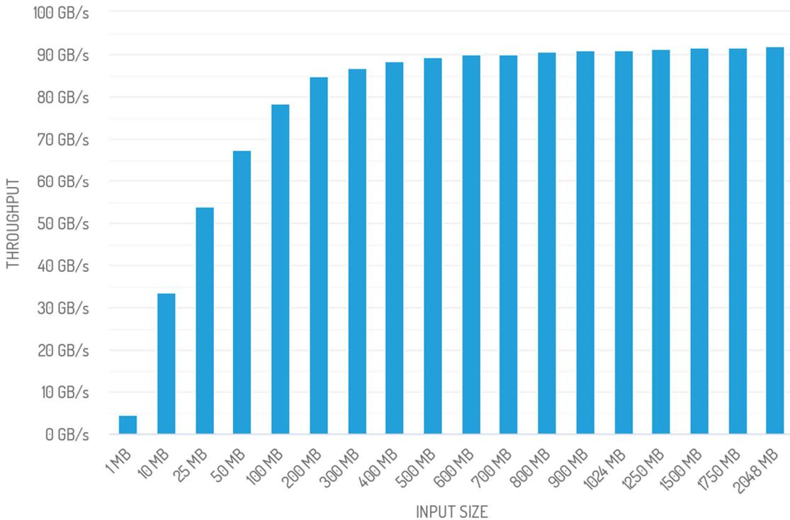
Figure 38: Performance scaling in relation to input size for *int\_444* on V100
