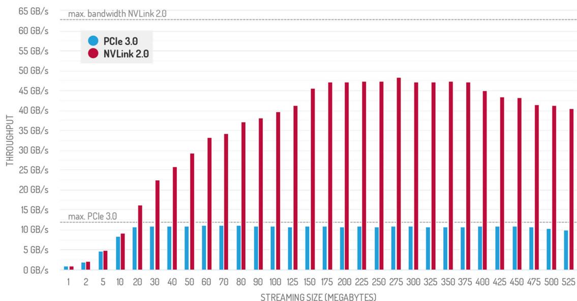
Figure 40: Impact of *streamingBatchSize* for *int\_444* on V100 over NVLink 2.0 in comparison
