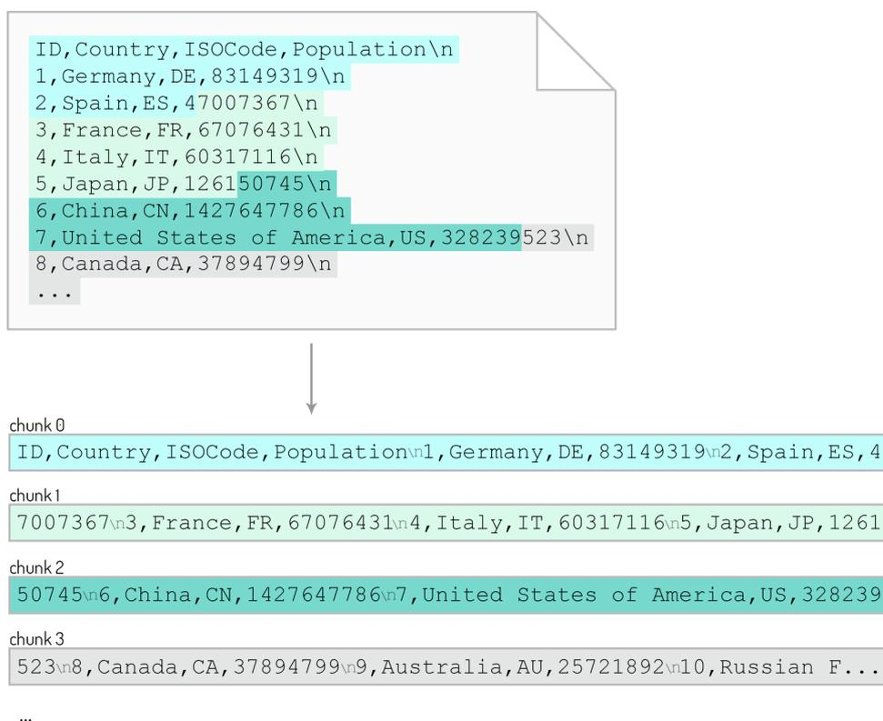
Figure 17: Splitting input into equally sized, independent, chunks
