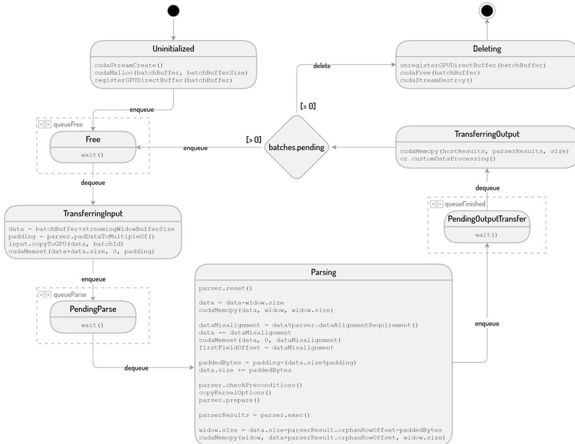
Figure 31: State diagram of a WorkStream item and the three WorkQueues
