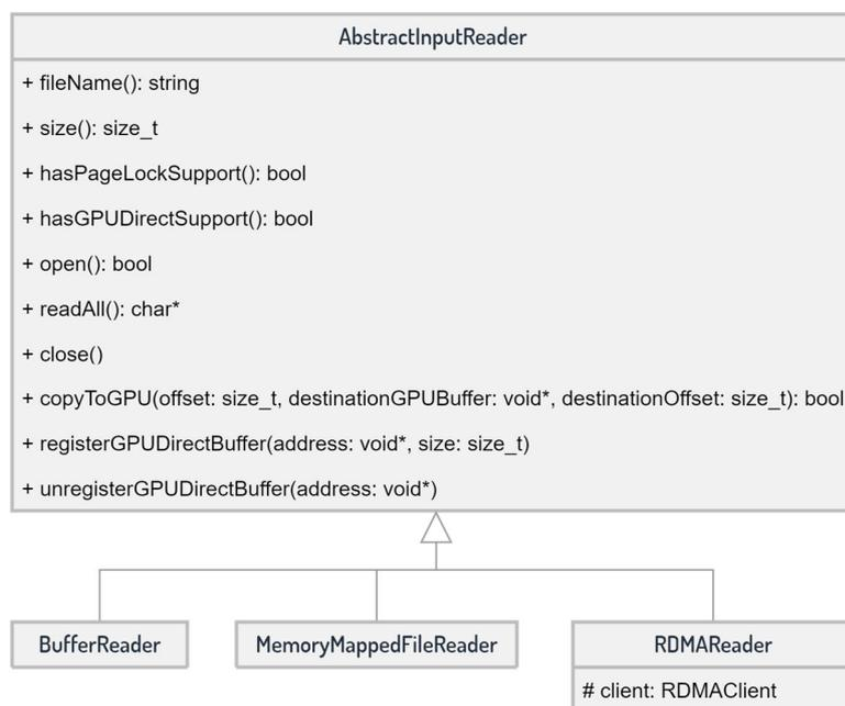
Figure 25: UML class diagram of input relevant components
