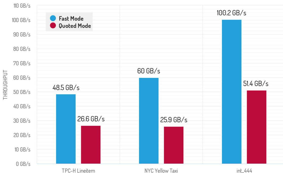
Figure 47: Comparison of Fast Mode and Quoted Mode on V100
