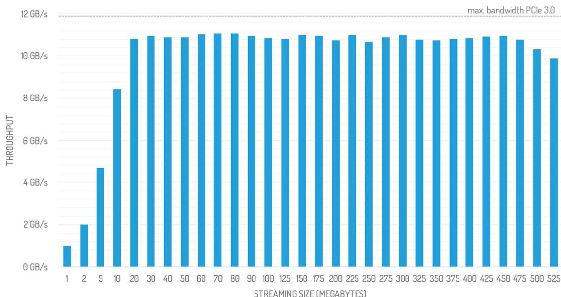
Figure 39: Impact of parameter *streamingBatchSize* for *int\_444* on V100 over PCIe 3.0
