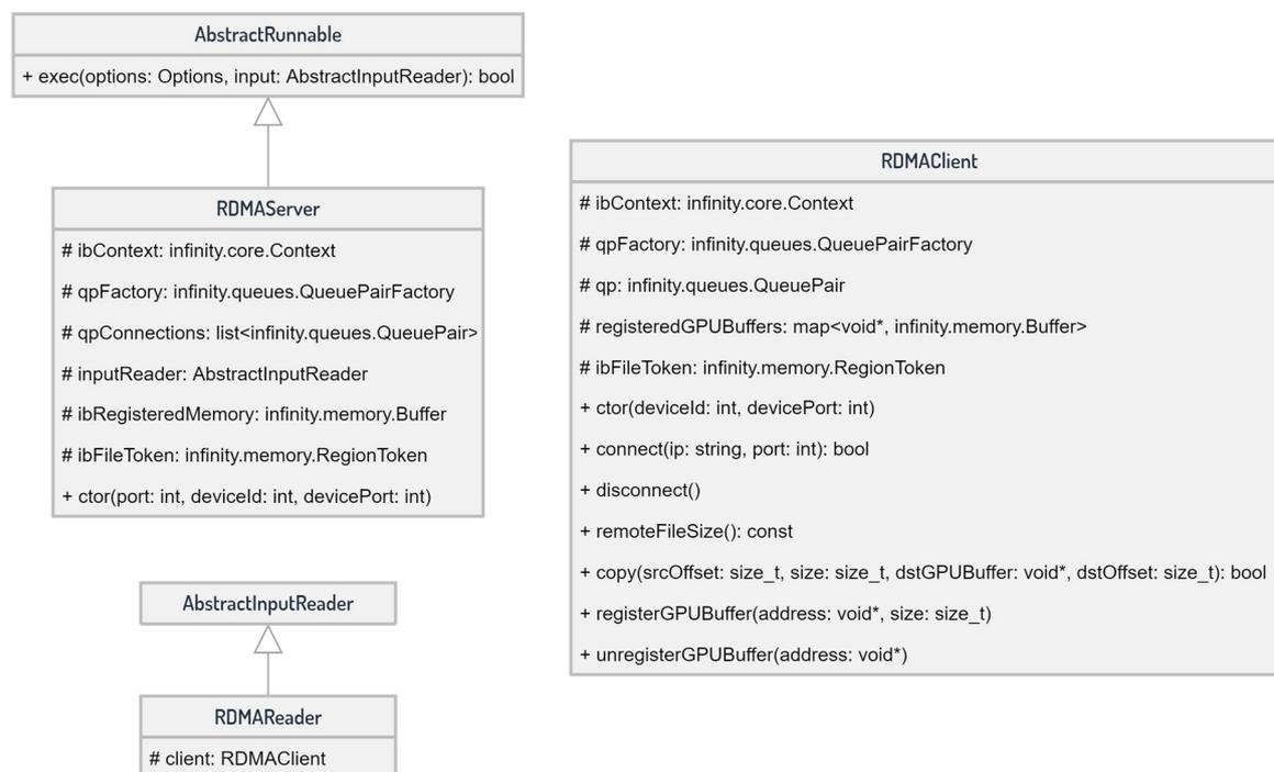
Figure 29: UML class diagram of RDMA specific components
