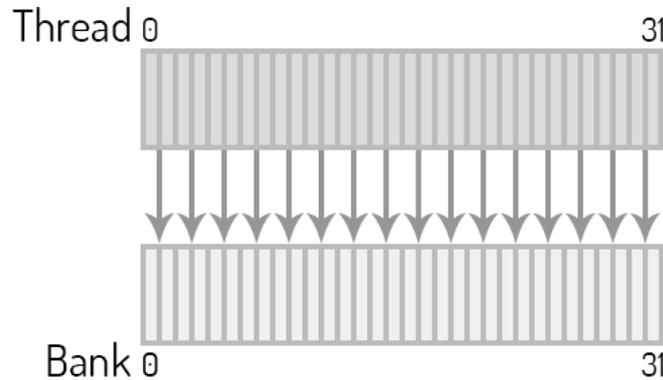
Figure 12: Optimal parallel access pattern. No bank conflicts, every thread accesses a different bank. Maximum bandwidth utilization.
