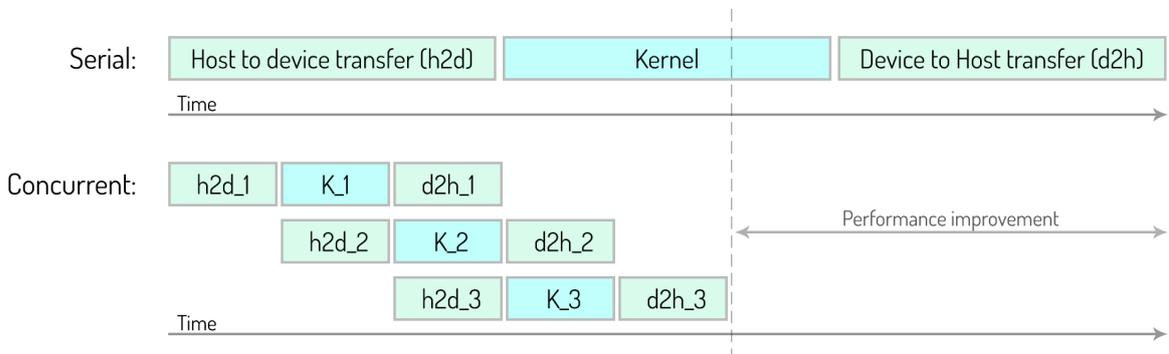
Figure 15: Example of using three CUDA streams to evenly distribute work
