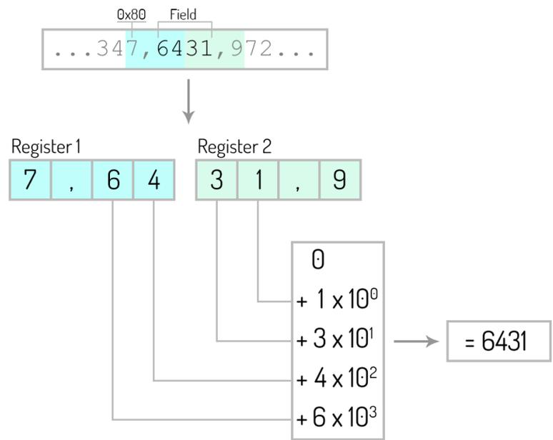
Figure 21: Thread reading aligned bytes to register for looped deserialization
