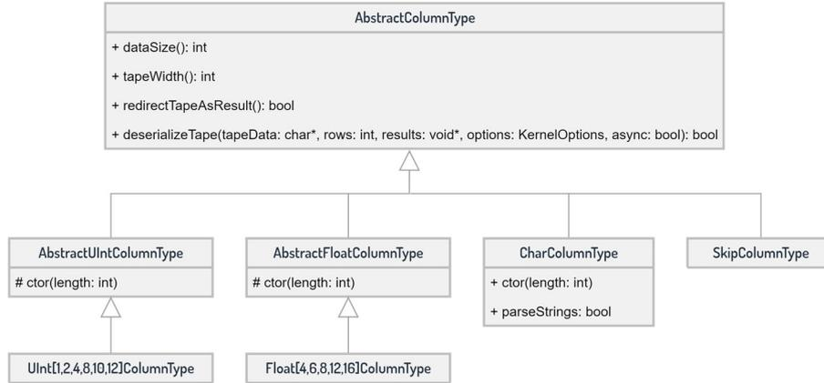
Figure 26: UML class diagram of deserialization relevant components
