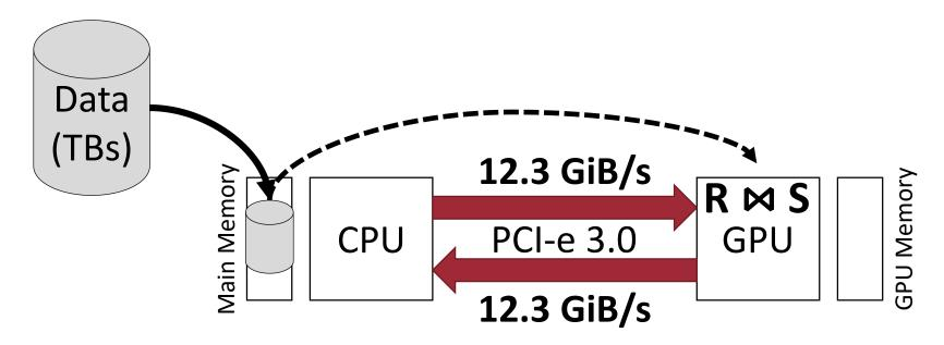
Interconnect bandwidth & GPU memory capacity limit scalability
