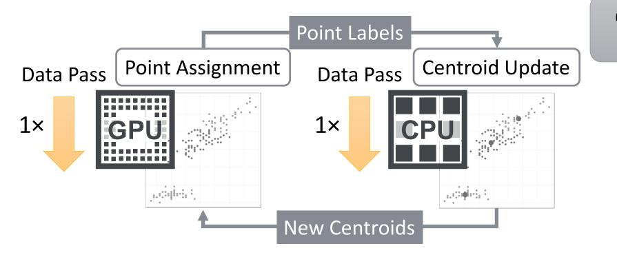
Offload compute intensive task to GPU
