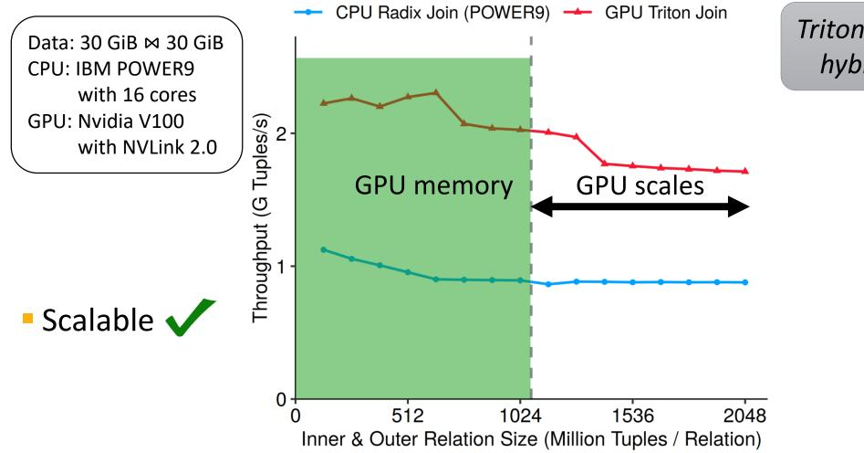
Triton join is new hierarchical hybrid hash join for GPUs
