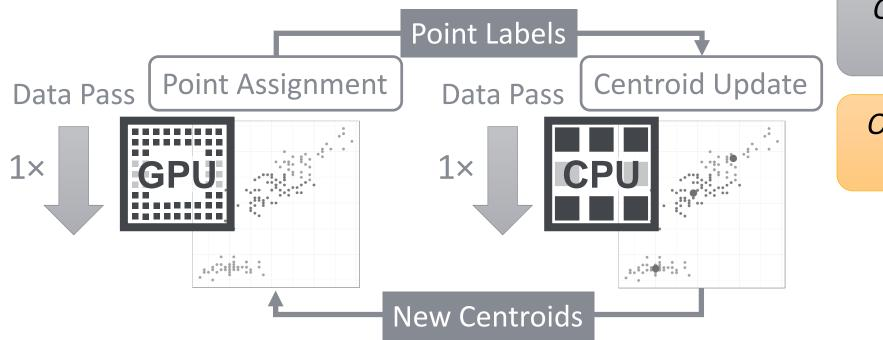
Offload compute intensive task to GPU
