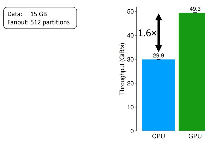
Exploit perfect coalescing using out-of-core partitioning
