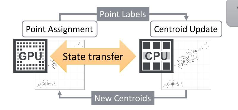
Offload compute intensive task to GPU
