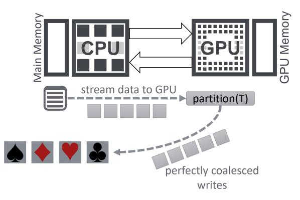
Exploit perfect coalescing using out-of-core partitioning
