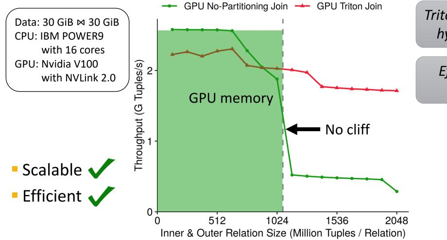
Triton join is new hierarchical hybrid hash join for GPUs
